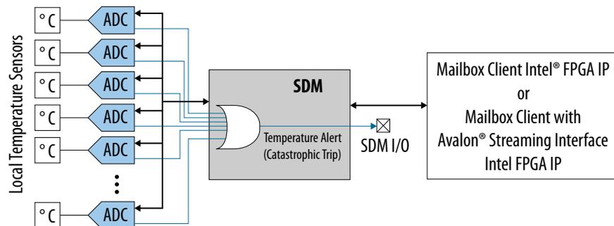
Intel Agilex 7 devices provide up to 11 local temperature sensor locations for monitoring on-chip temperature.
