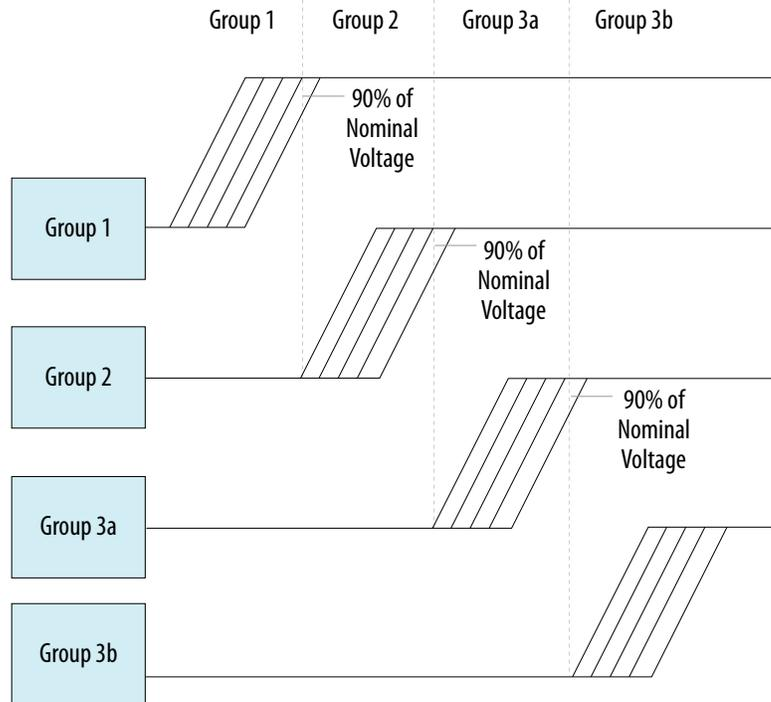
**Note:**  $V_{CCBAT}$  is not in any of the groups below.  $V_{CCBAT}$  does not have any sequence requirements.  $V_{CCBAT}$  holds the content of the security keys.
