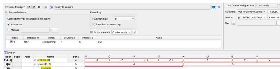
7. In the **In-System Sources and Probes Editor** window, verify that the **probe[4..0]** signal is toggling.
