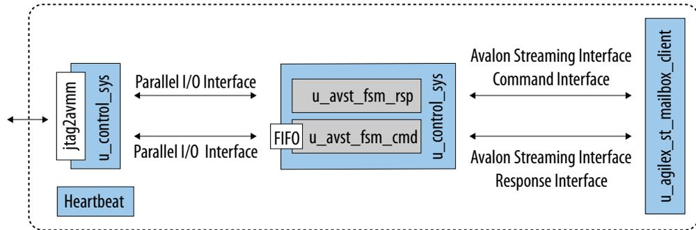
All the Intel Quartus Prime System Console read and write commands control a set of parallel I/O IPs that select a command for the Mailbox Client with Avalon Streaming Interface IP to execute. At the same time, the parallel I/O IPs control a FIFO IP that stores all the Mailbox Client with Avalon Streaming Interface IP responses.
