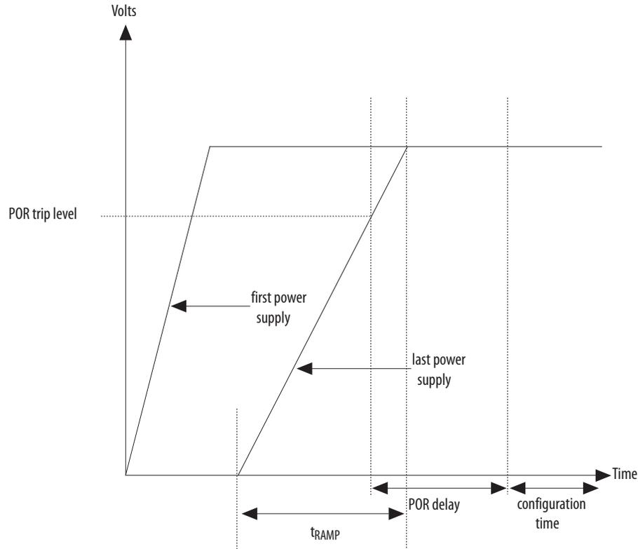
The Intel Agilex 7 POR circuitry uses individual detection circuitry to monitor each of the configuration-related power supplies independently. The POR circuitry is gated by the outputs of all the individual detectors.
