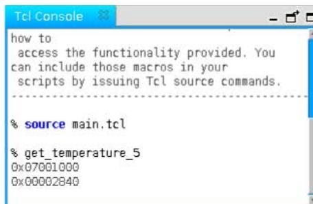
The System Console displays the results after the command. The first element of the results represents the header of the Mailbox Client with Avalon Streaming Interface IP response.
