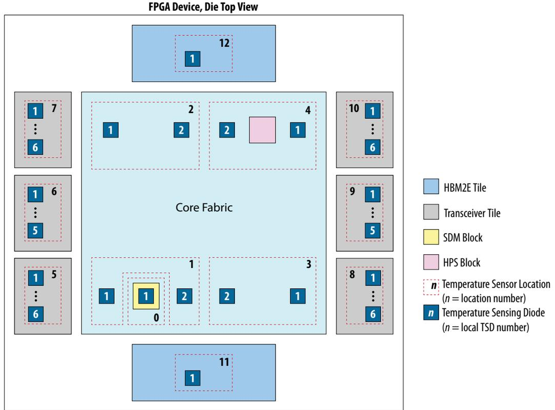
**Note:** Availability of the transceiver tiles varies among different Intel Agilex 7 series, densities, and packages. The HPS block is only available in Intel Agilex 7 SoC FPGAs. The HBM2E tiles are only available in M-Series FPGAs.
