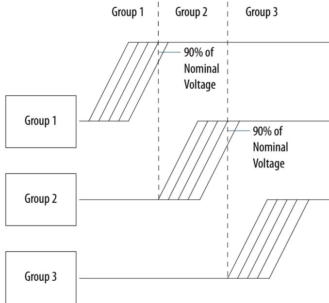
The following figure shows the voltage groups of the Intel Agilex 7 M-Series devices and their required power-up sequence.
